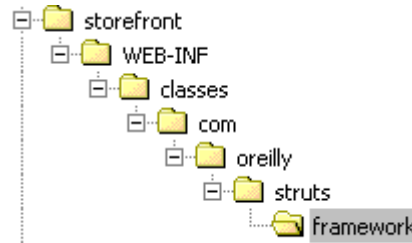
Figure 4-2. Java classes that are in a package must be in the proper directories
